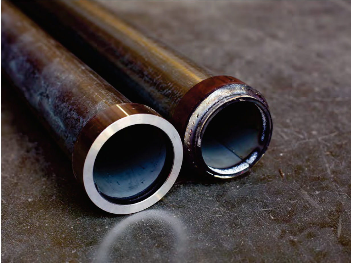
Figure 2.9 PP288 starter tubes with pressed fit and welded friction reduction collars
